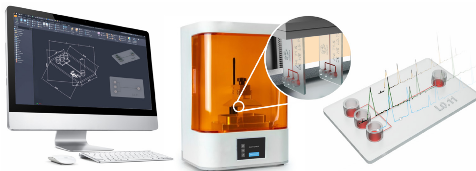
Figure 1. Schematic illustration of the 3D-printing fabrication process of an AMD.
