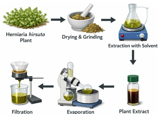
Figure 2. Schematic illustration of the extraction process of the Herniaria hirsuta plant.
