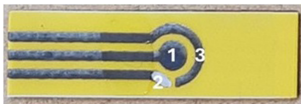
Figure 1. Image of the LIG-based device fabricated on a polyimide tape, comprising (1) a working electrode, (2) a pseudo-reference electrode, and (3) a counter electrode.
