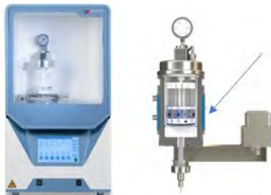
Figure 2: UW3 microwave digestion system with focus on the SRC chamber
