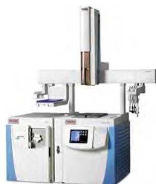
Figure 2. ISQ GC-MS system with TriPlus RSH autosampler.
