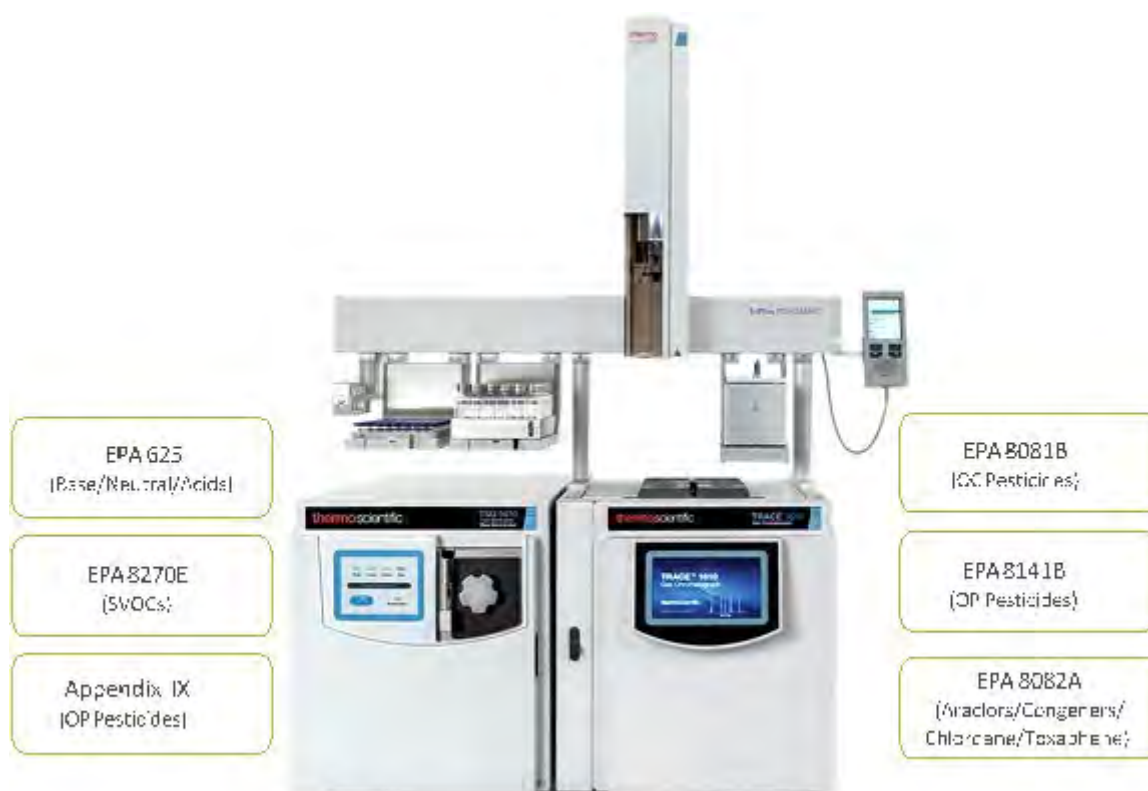
Figure 1. Unified environmental method schematic for analysis of multiple compound classes using a single analytical platform.
